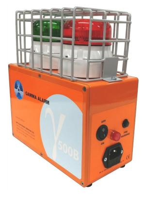
The 500B GAMMA-ALARM is a portable, battery powered alarm system designed for Gamma-ray inspection areas utilizing an internal GM tube. The alarm will indicate audibly before and visually when an exposure is in progress. The pre-set threshold level is typically 7.5 $\mu$ Sv/h unless otherwise specified. The 500B GAMMA-ALARM can also be used anywhere in the world as it can accommodate a supply voltage from 100V AC to 240V AC 50/60Hz.
